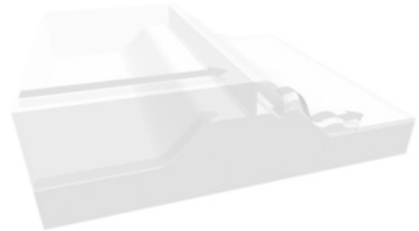
Erosion by water after overtopping
