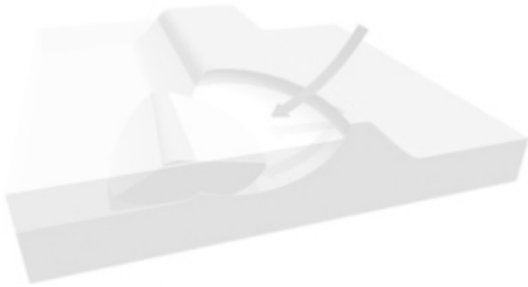
Lateral instability due to effects of water on soils
